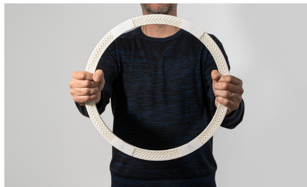
LCM-printed ALD ring with 15" diameter printed by Alumina Systems
